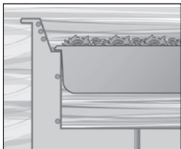
The unique angled inside wall design provides easy access and clear views. The greater surface area of the angled wall and the placement of the coils allow cold air to more effectively blanket your food product.
